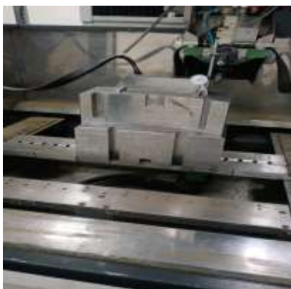
EDM Die Sinking on Main Block Slider Part
