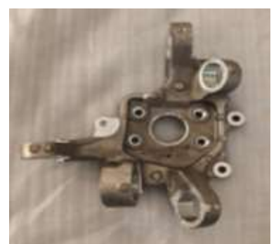
Steering Knuckles Machining for TATA ROWA Project on CNC 5 Axis Milling Machine
