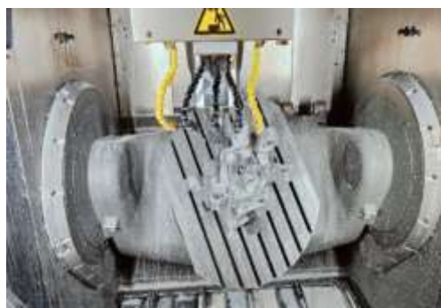
Steering Knuckles Machining for TATA ROWA Project on CNC 5 Axis Milling Machine
