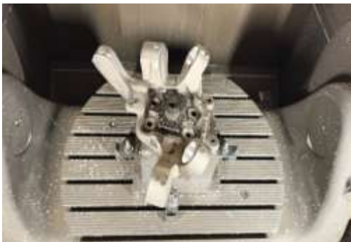
Steering Knuckles Machining for TATA ROWA Project on CNC 5 Axis Milling Machine
