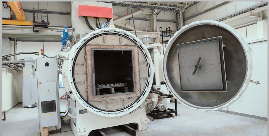
VACUUM HEAT TREATMENT FURNACE -01 NOS
